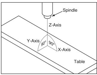
**Figure 69.** Spindle Z-axis perpendicular to the table X- and Y-axis.
